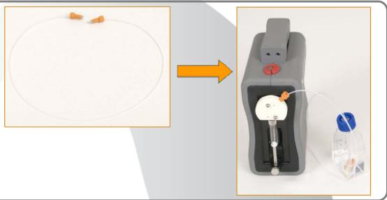
2. Connect outlet cable as shown.
