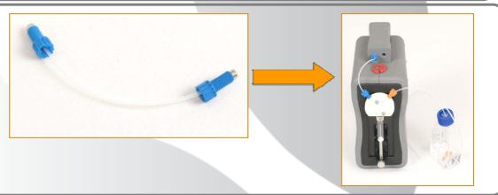
**3.** Connect cable to MultiFlow8 as shown.
